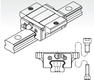
This type offers the installation either from top or bottom side of carriage.
