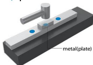
Continue pounding the cap until the cap is on the same plane with the top surface of rail.
