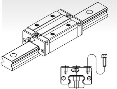
All dimensions are same as SME-SA except the mounting hole dimensions of carriage are different and the height is lower, which do not change the basic loading rating.
