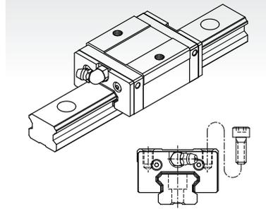
Square type with smaller width and can be installed from top side of carriage.
