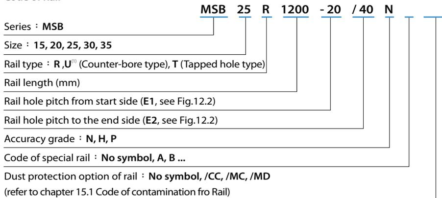
Notr<sup>(1)</sup> : U type rail is only applicable for MSB15 with M4 mounting hole.
