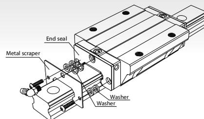
Removing spatters, iron chips, and large foreign matters as well as protecting the end seals.
